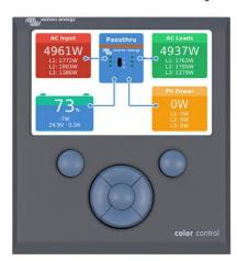
Color Control panel, showing a PV application
